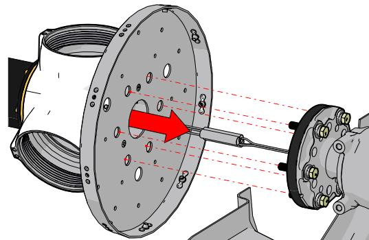
(iii.) Non-fitted spacer assembly ( $< 0.75\text{in}$ ) with mini slings assembly.
